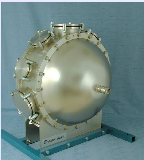
Double-wall reaction vacuum chamber for experiments with cryogenic tritium target-FLNR
