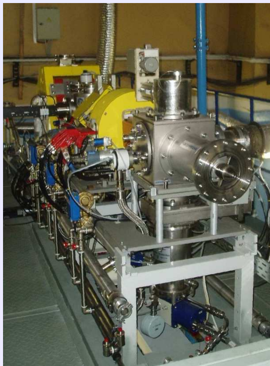
Upgrade of the IC100 vacuum system
